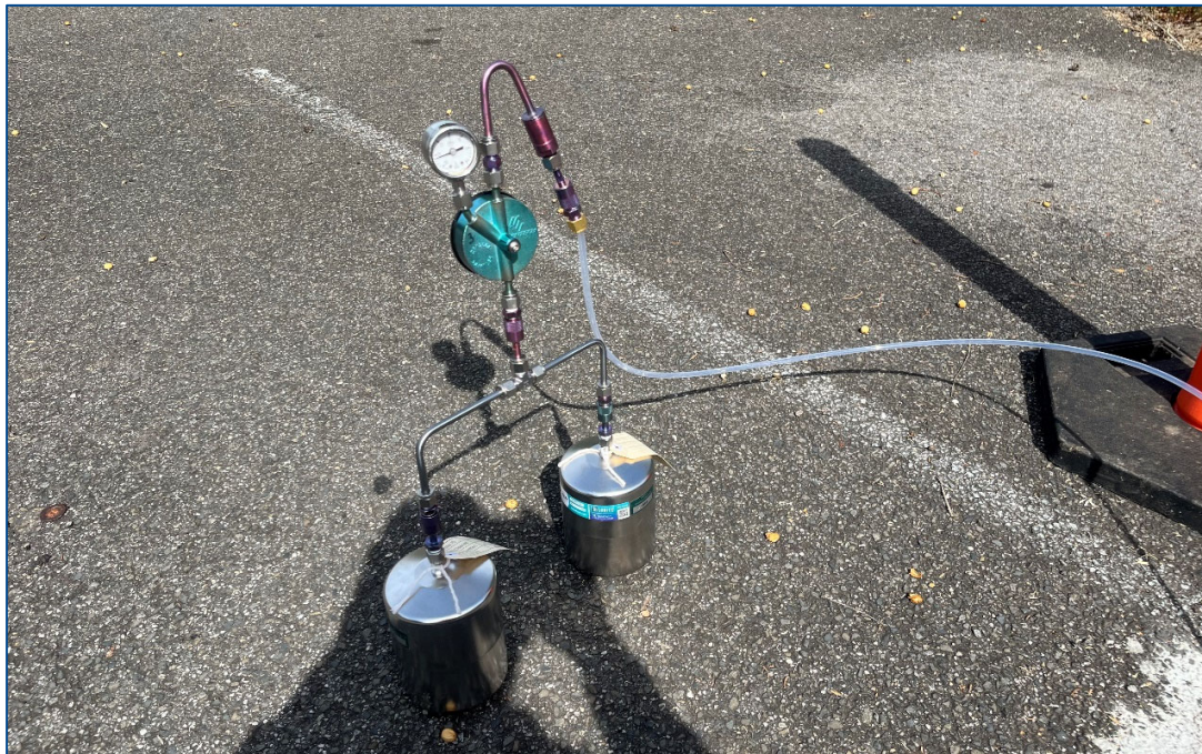
Photograph 8: View of the soil vapour sampling set-up for soil vapour sample well SV04 and duplicate sample SV_QC03.
