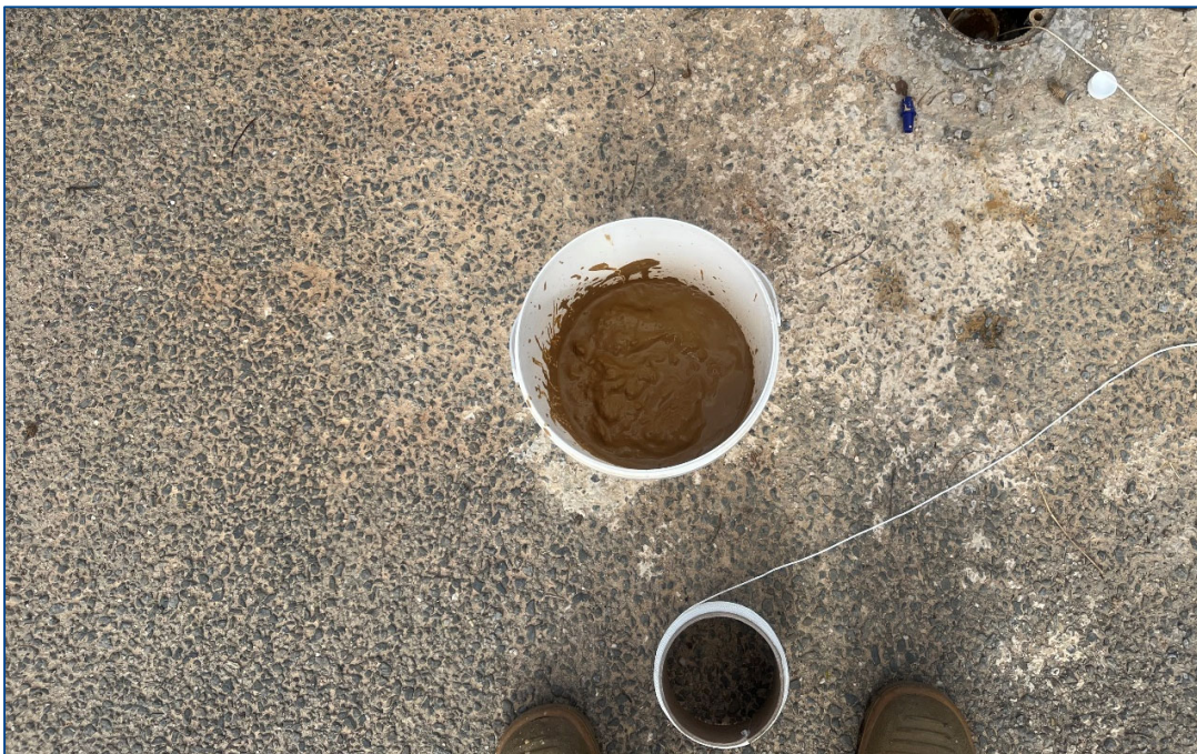
Photograph 6: Each newly installed wells was found to require further redevelopment due to stratification of silts within the water column. Following redevelopment, wells were resampled.
