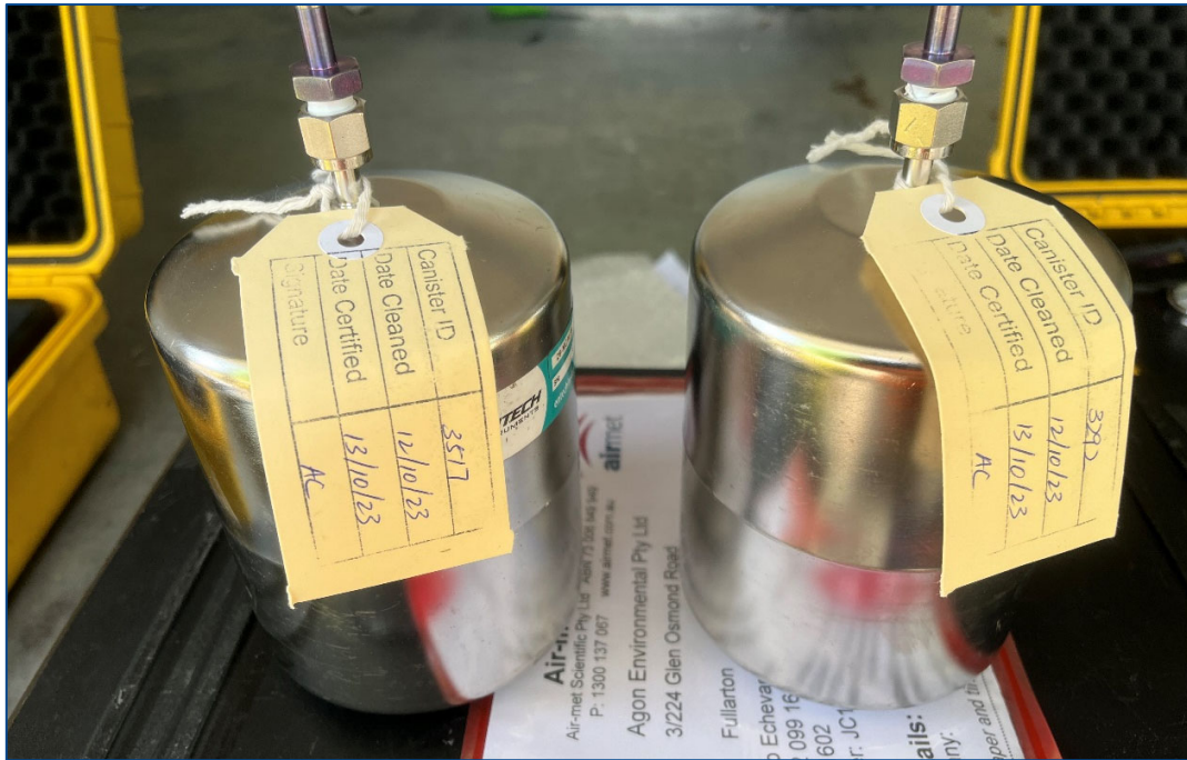
Photograph 7: Summa Canisters were checked for leaks using an analogue vacuum gauge .
