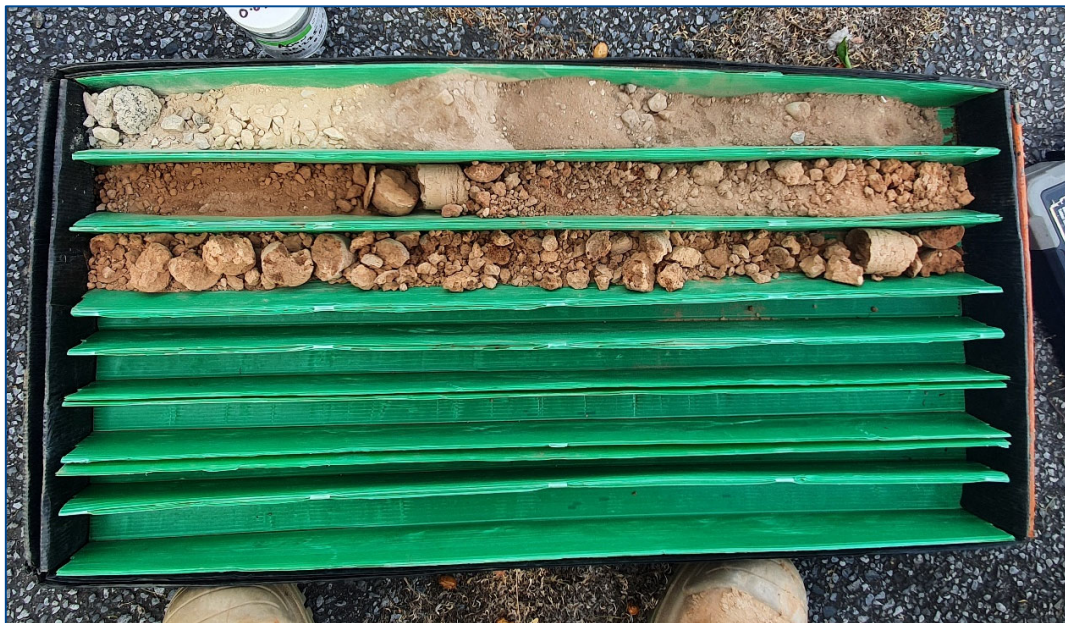
Photograph 4: View of soils from A-BH01. Soil at and adjacent this bore location has since been excavated to a depth of 0.5 following the discovery of fill soils with elevated benzo(a)pyrene concentrations.
